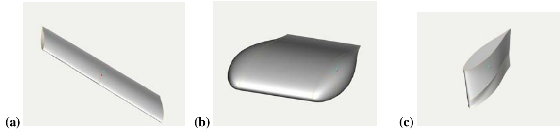
Figure 15. Components of the twin H-body configuration, (a) cross-foil, (b) H-body, and (c) strut.
