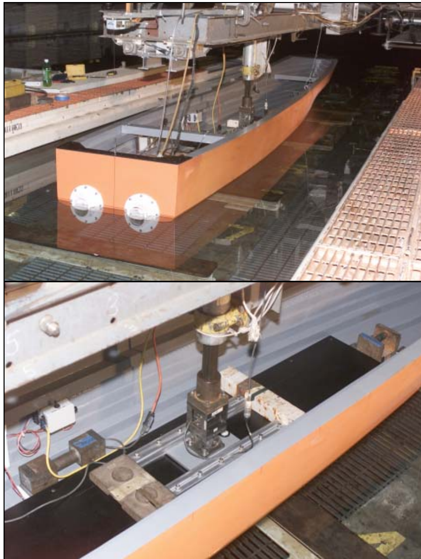
Figure 4. Waterjet Self-Propulsion Towing Arrangement
