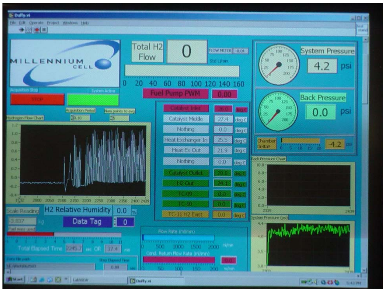
Figure 2.3: Bench test computer display of the control and data acquisition interface for the HOD™ system.
