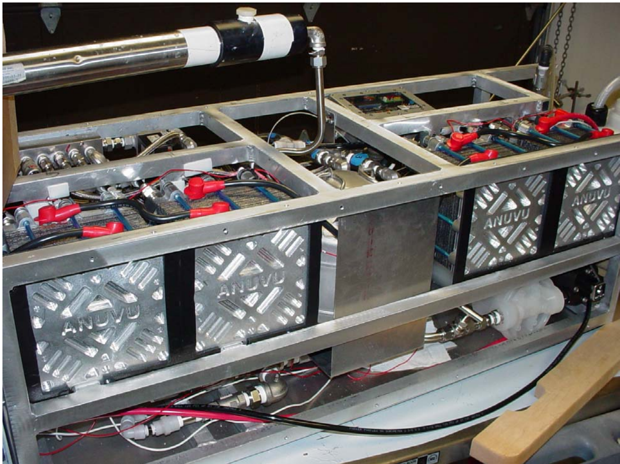
Figure 2.1: Front view of the Anuvu Fuel Cell Products Proton Exchange Membrane 3 kW (net) fuel cell system at the Millennium Cell facility in Eatontown, NJ.
