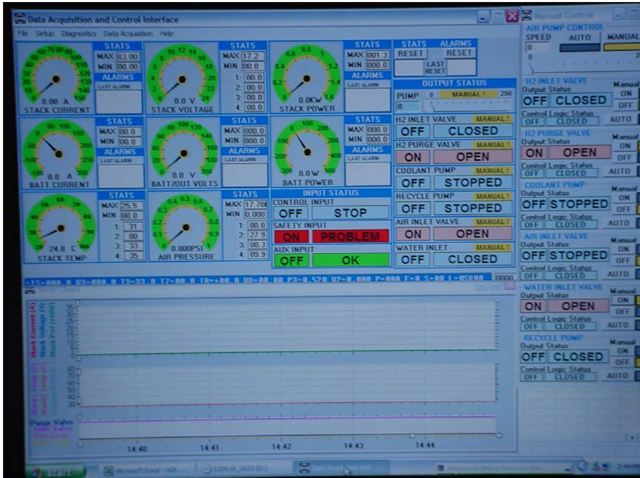
Figure 2.2: Bench test computer display of the control and data acquisition interface for the fuel cell system.
