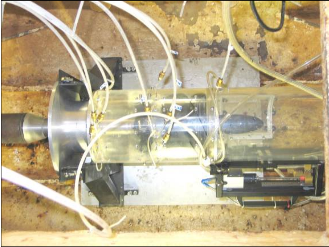
Figure 7. Laser Apparatus Mounted to the Inlet Duct in the Lower Right-hand Corner
