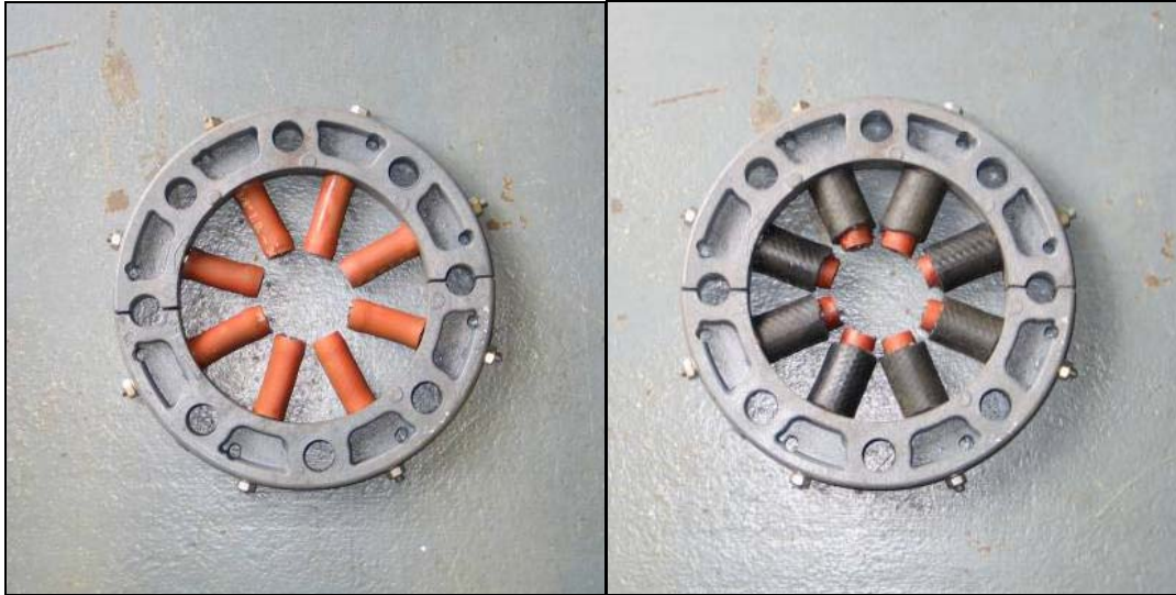
Figure 8. Flow Restrictor with Low Blockage (left) and High Blockage (right)
