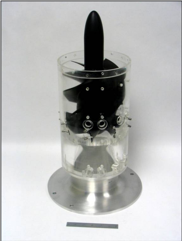
Figure 2. Stack-up of Pump Model Components on the Stator Adaptor
