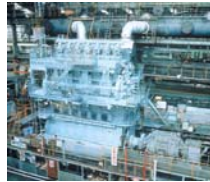
Sulzer low-speed RTA and RT-flex engine 80 MW.
