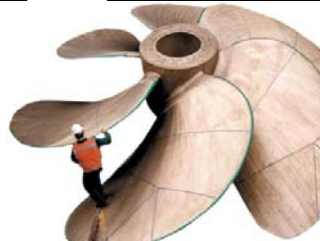
World's Largest Fixed Pitch Propeller 66 mW - 94.5 Ton
