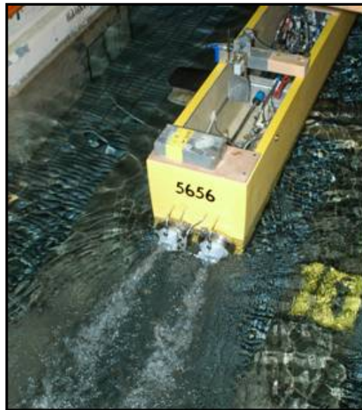
Figure 11: Self-Propulsion Model in the Towing Tank
