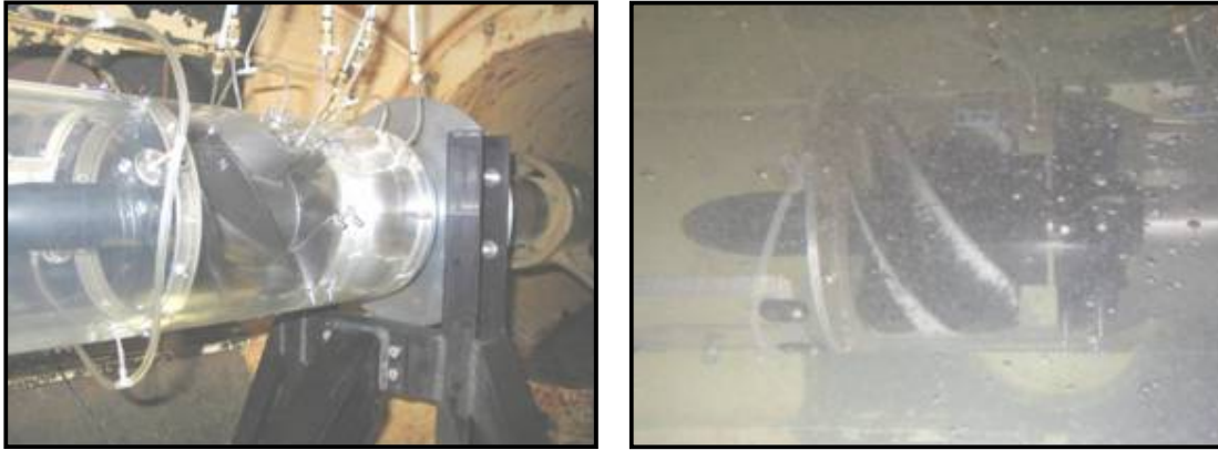
Figure 10: Cavitation run at 2000 rpm and Q/Q_d = 1.0
