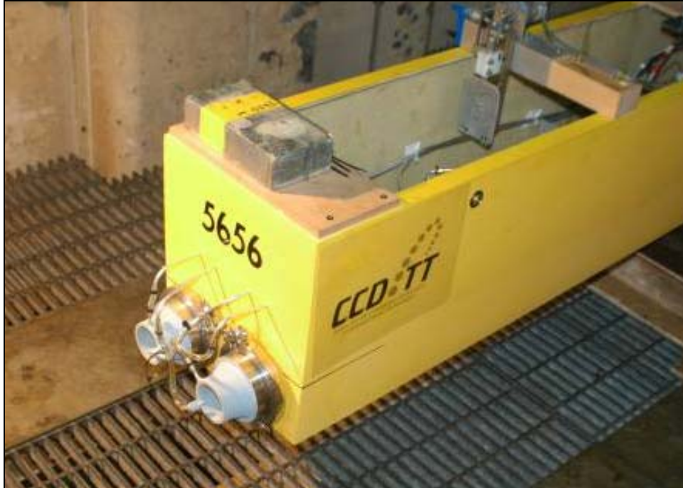
Figure 17. Later View of the Model with Transom and Waterjets Installed
