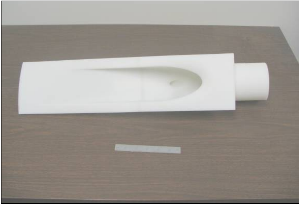
Figure 4. Model Waterjet Inlet Opening in the Hull
