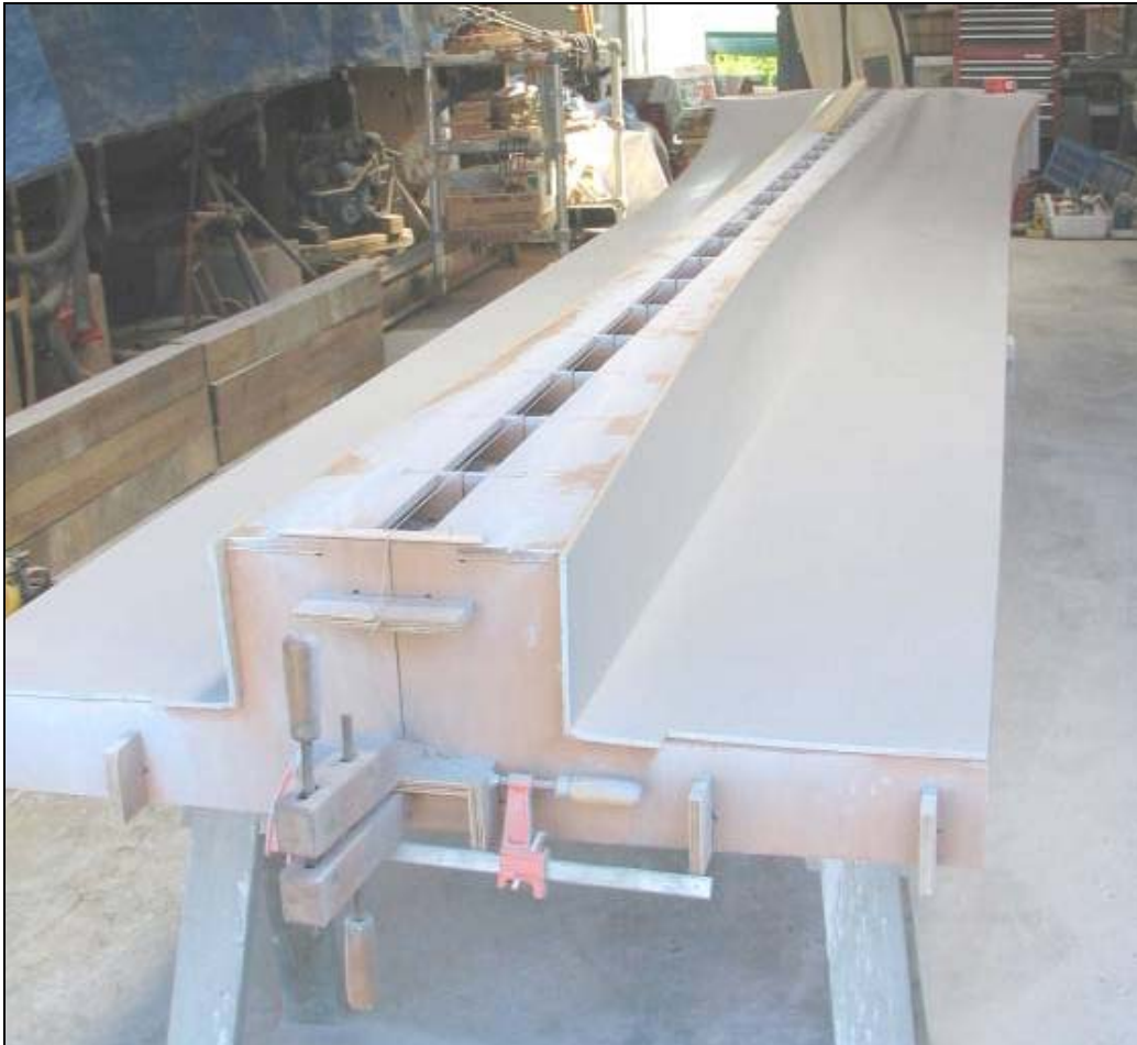
Figure 13. Two Mold Sections for Building the Model Halves
