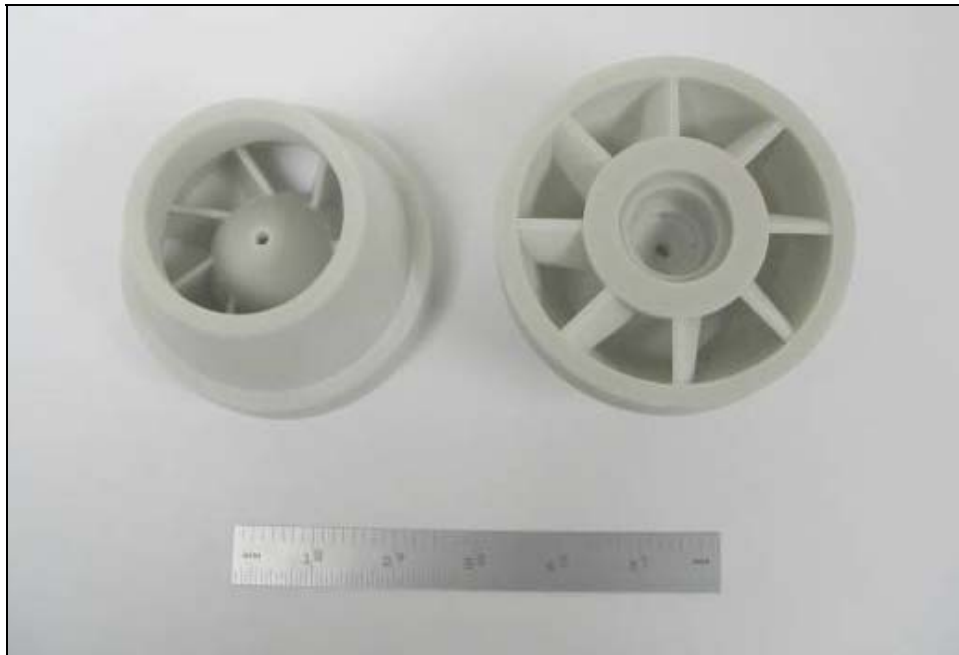
Figure 8. Front and Rear View of the Stator-Nozzle Section
