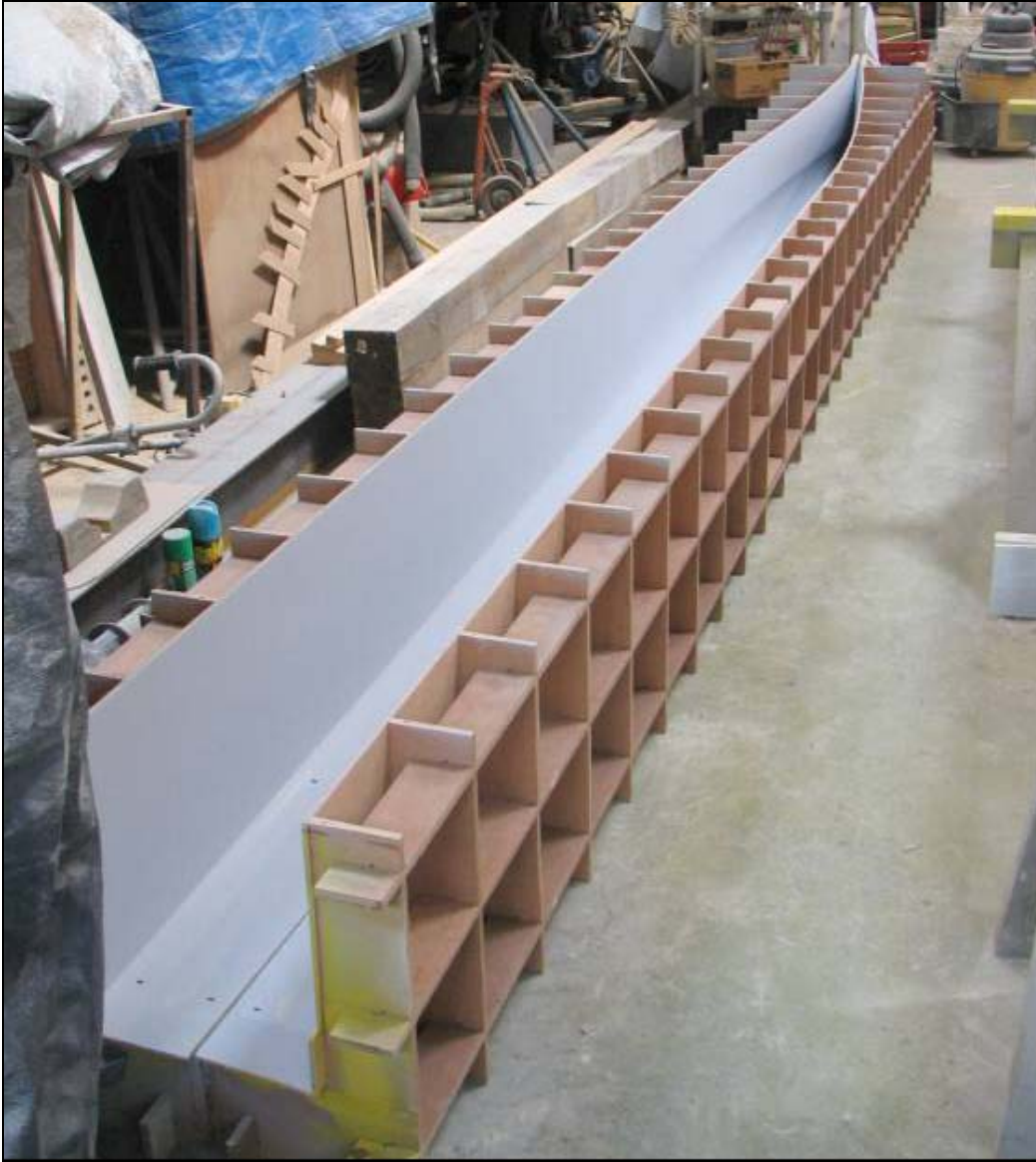
Figure 14. Egg Crate Arrangement of the Mold Frames Arranged for Alignment Check
