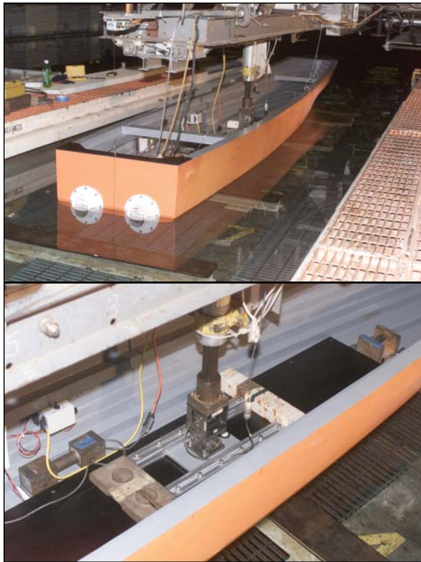
Figure 4. Waterjet Self-Propulsion Towing Arrangement
